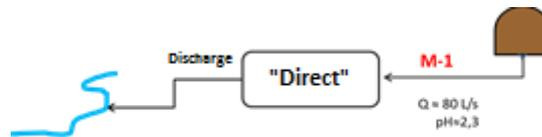
**Figure 3.** Typical scheme of a processing system using direct neutralization.
