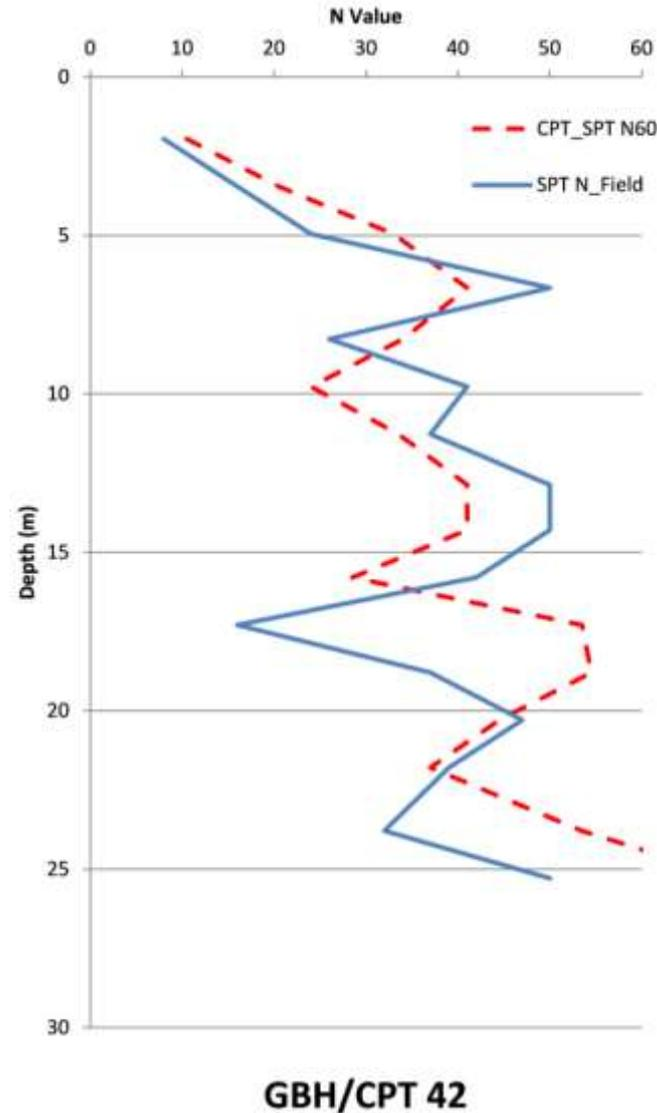
Figure 1. Graphical comparison of CPTu derived SPT  $N_{60}$  with SPT  $N_{field}$  Values-Test location No. 42.
