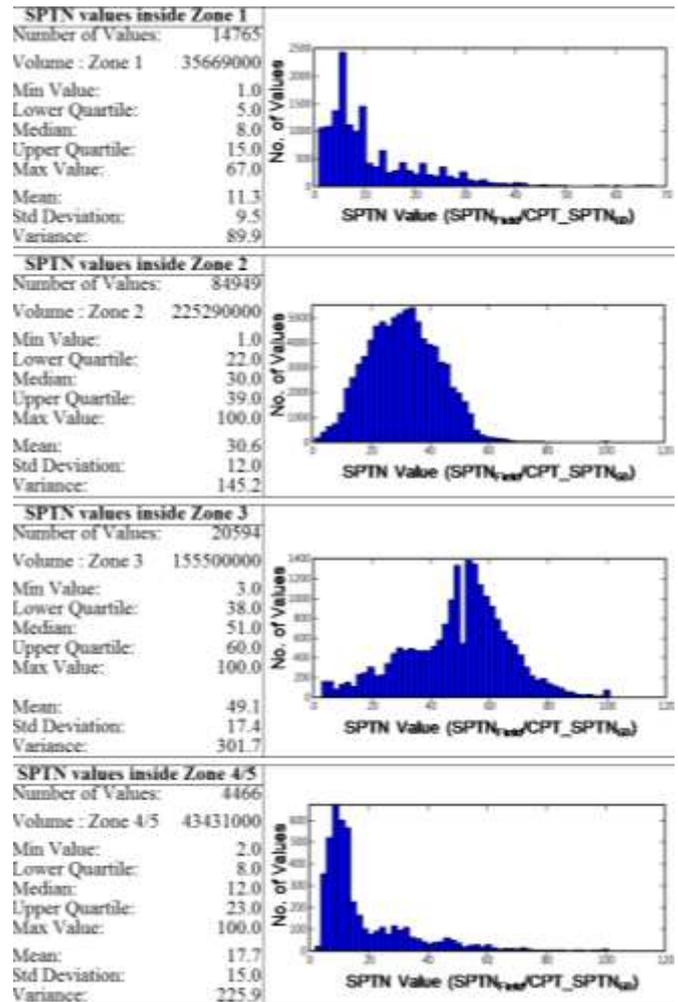
It is therefore clear from the data evaluation shown in Table 4 that the numerical data and the zone model has been successful in delineating distinct geotechnical zones that can be applied to the mine planning and design process.
