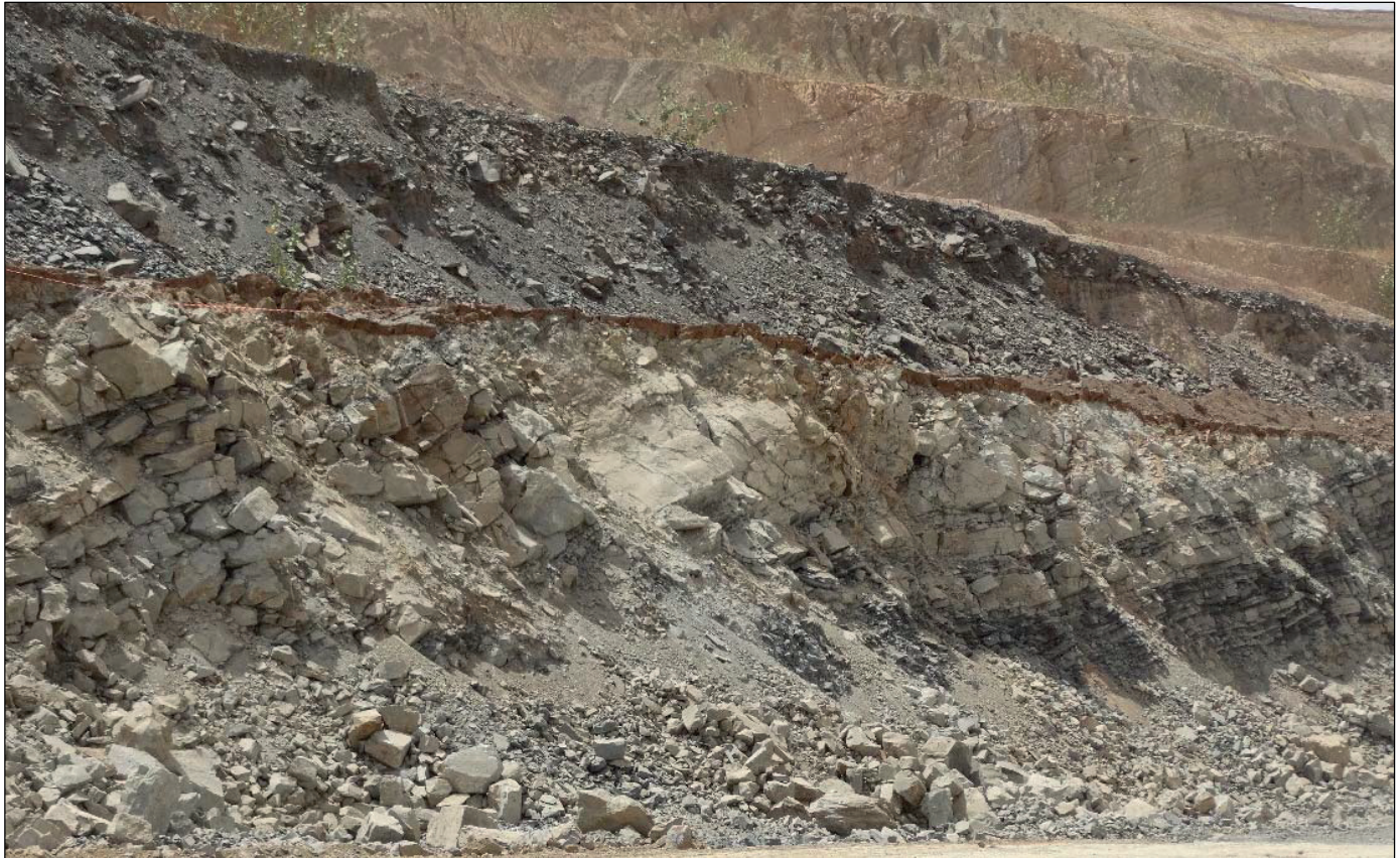
Figure 4: Transition Rock Materials exposed across a recently blasted Bench Slope
