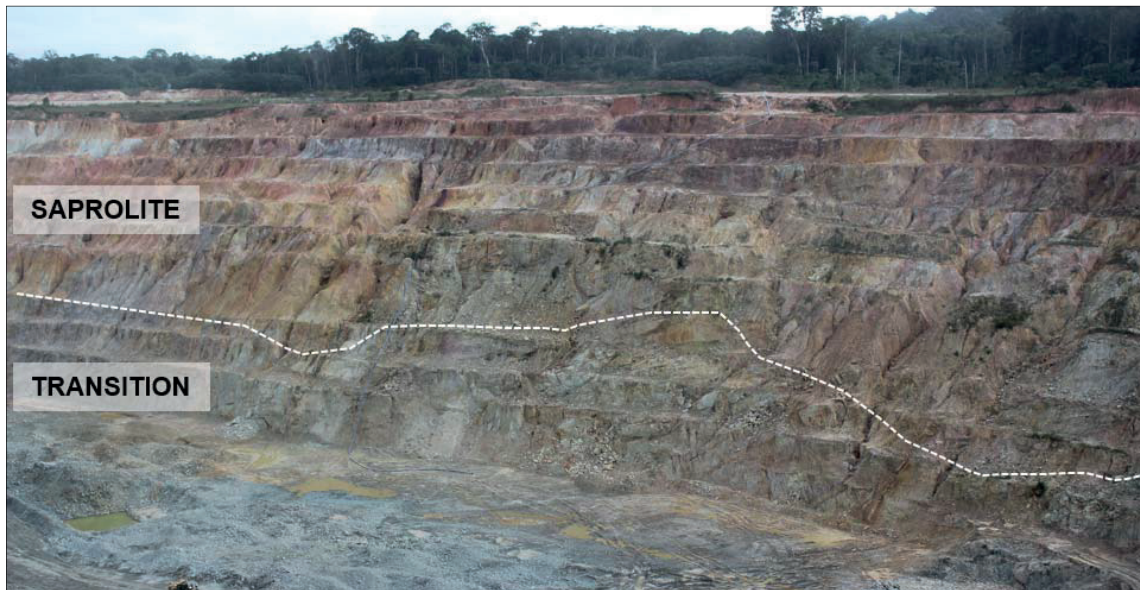
Figure 10: Weathered Rock Profiles across the South Wall, Rosebel Pit
