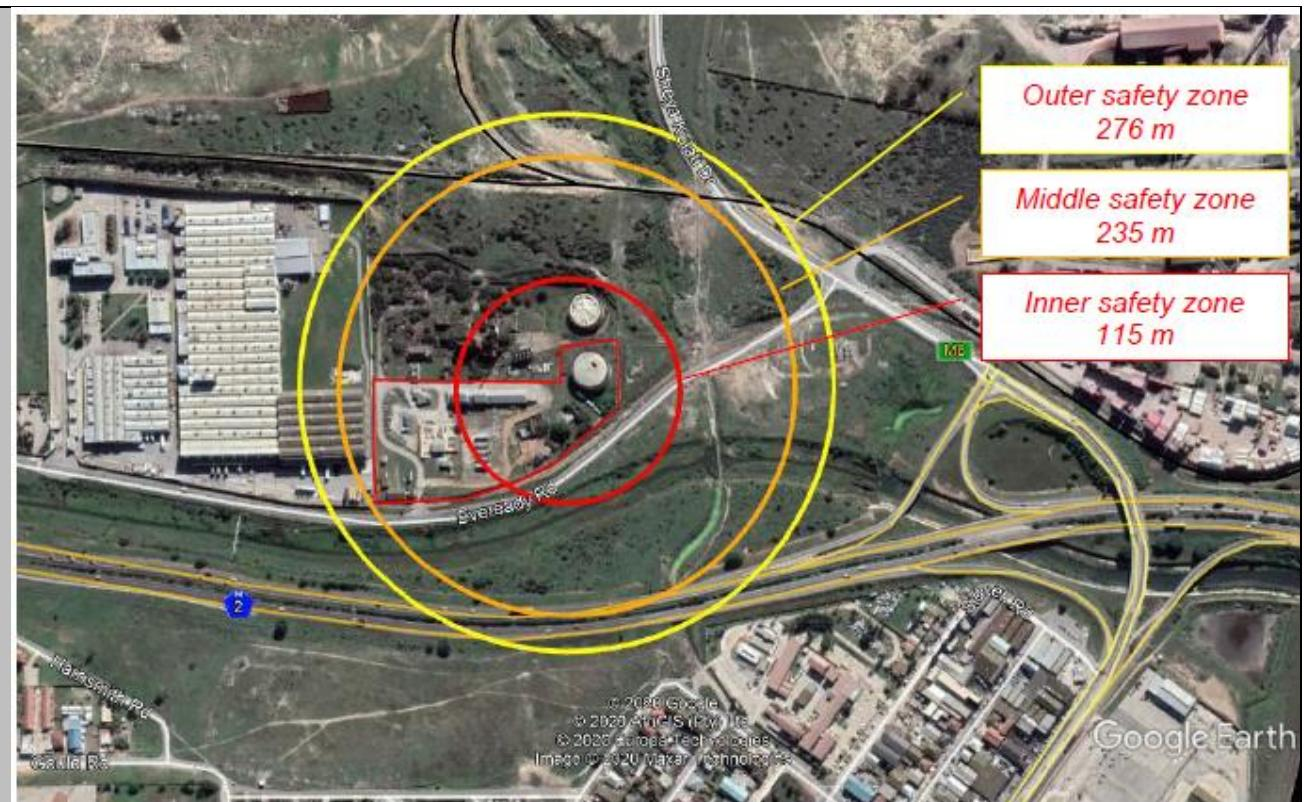
**Figure 1: Safety Risk isopleth map for the site, including the new proposed 400 m<sup>3</sup> tank**
