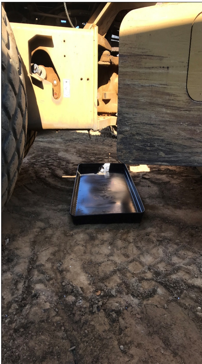
Plate 1: Drip trays placed under all plant in the construction camp
