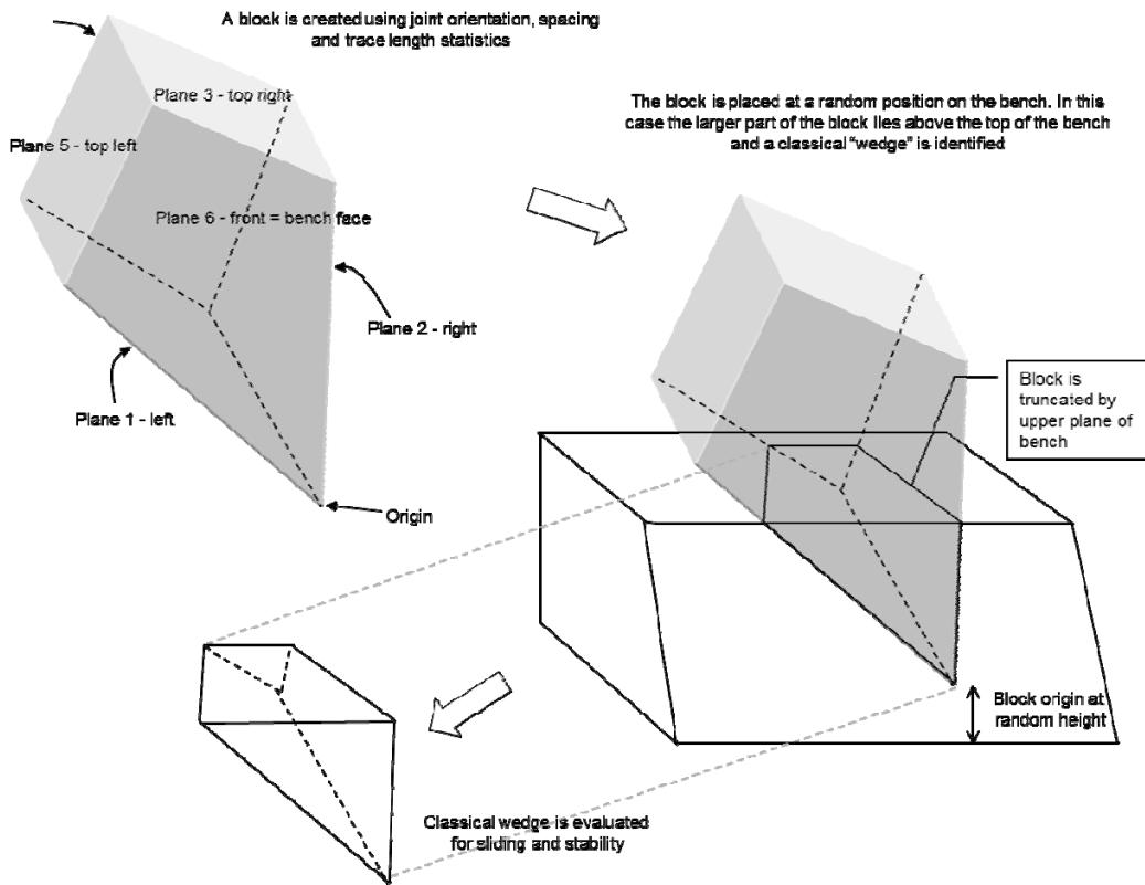
**Figure 3** Example showing how a classic wedge shaped block may be formed.
