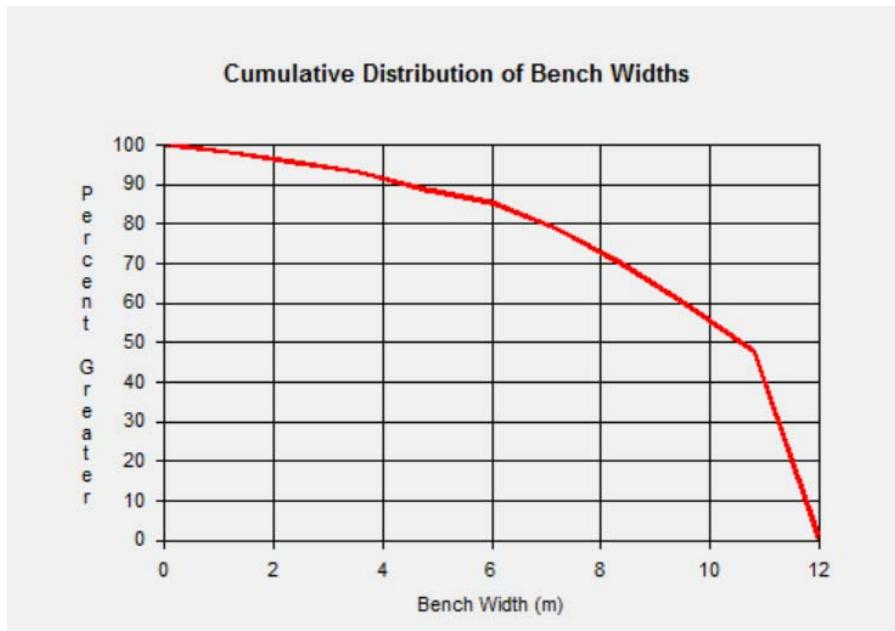
**Figure 7** Cumulative distribution of bench widths for berms that were originally 12 m wide. The figure shows, for example, that 80% of the benches are greater than 7 m wide.
