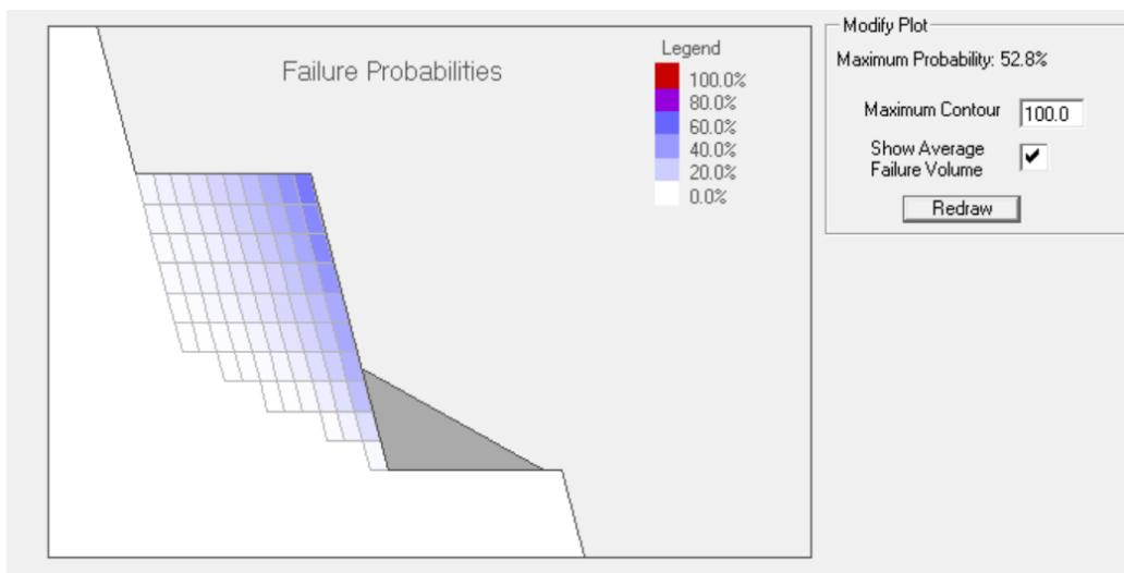
**Figure 6** Depth of failure of a bench expressed as a probability of failure. The figure shows that there is a 53% probability that the crest will be failed and the probability drops to about 20% at a depth of 6 m. It also shows the pile of rubble that will form at the toe of the slope – based on the average volume of failure. This shows that the bench effectiveness is reduced by about 95%.
