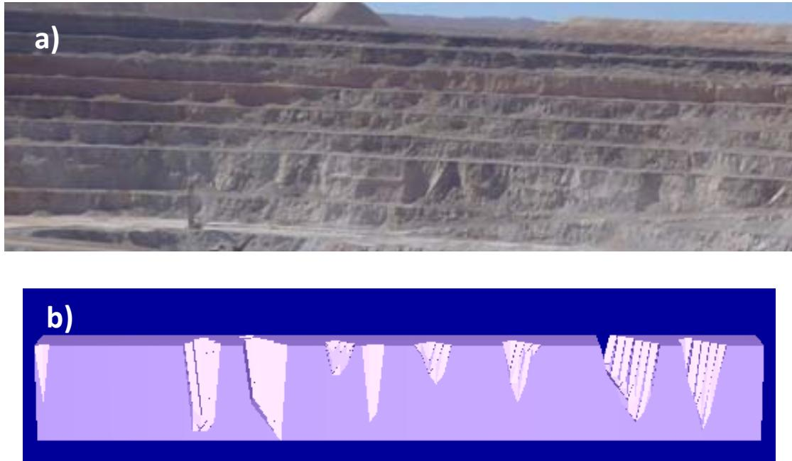
**Figure 11** Calibration on site of bench berm analysis. (a) Picture of the slopes benches in the structural domain. b) Output of SBlock program showing the failed blocks removed (red zones) for this sector using structural domain data shown in Table 3.
