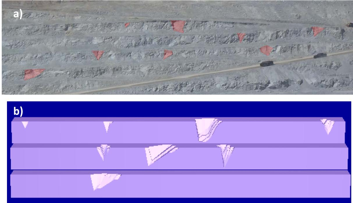
**Figure 10** Calibration on site of bench berm analysis. (a) Picture of the slopes benches in the West wall, Structural Domain A. b) Output of SBlock program showing the failed block removed (red zones) for this sector using structural domain data shown in Table 2.
