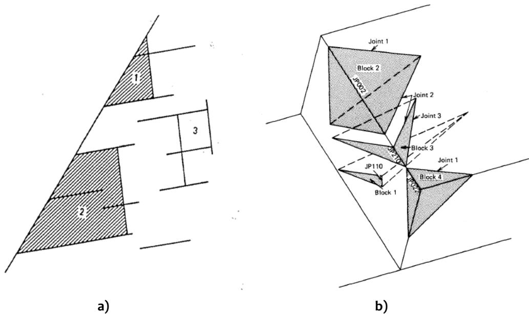
**Figure 1** Some types of blocks in a rock slope. a) Types of blocks in a slope: (1) key blocks; (2) removable blocks with parallel faces; (3) joint blocks. b) Removable blocks in a rock slope.
