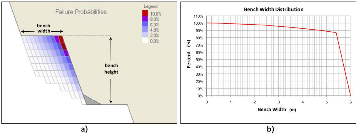
**Figure 9** Output of SBlock program showing the probability of failure expressed as a depth of failure of a bench applied to the southeast sector of “Carmen de Andacollo” final pit (a). Cumulative distribution of bench widths for the southeast sector of “Carmen de Andacollo” final pit (b).
