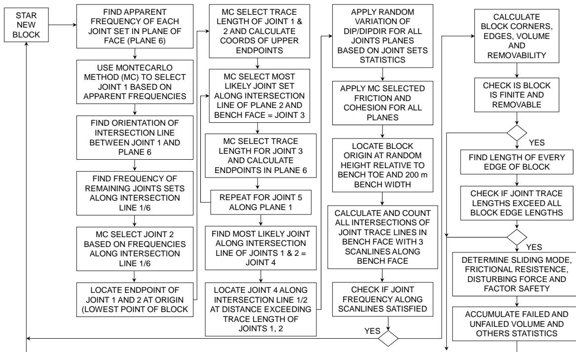
**Figure 2 Flow chart for block formation from trace length and orientation statistics.**
