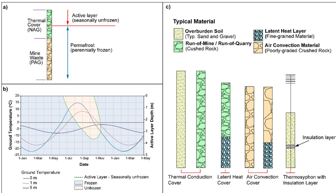
Figure 1. a) Schematic diagram of a thermal cover, b) typical progression of active layer and near surface ground temperatures for one year, and c) basic types of thermal covers.
