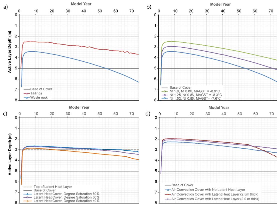
Figure 3. Estimated active layer depth for a) thermal conduction covers underlain by waste rock and tailings, b) thermal conduction covers with varying ground surface temperature, c) latent heat covers with varying material saturation, and d) air convection covers with and without a latent heat layer.
