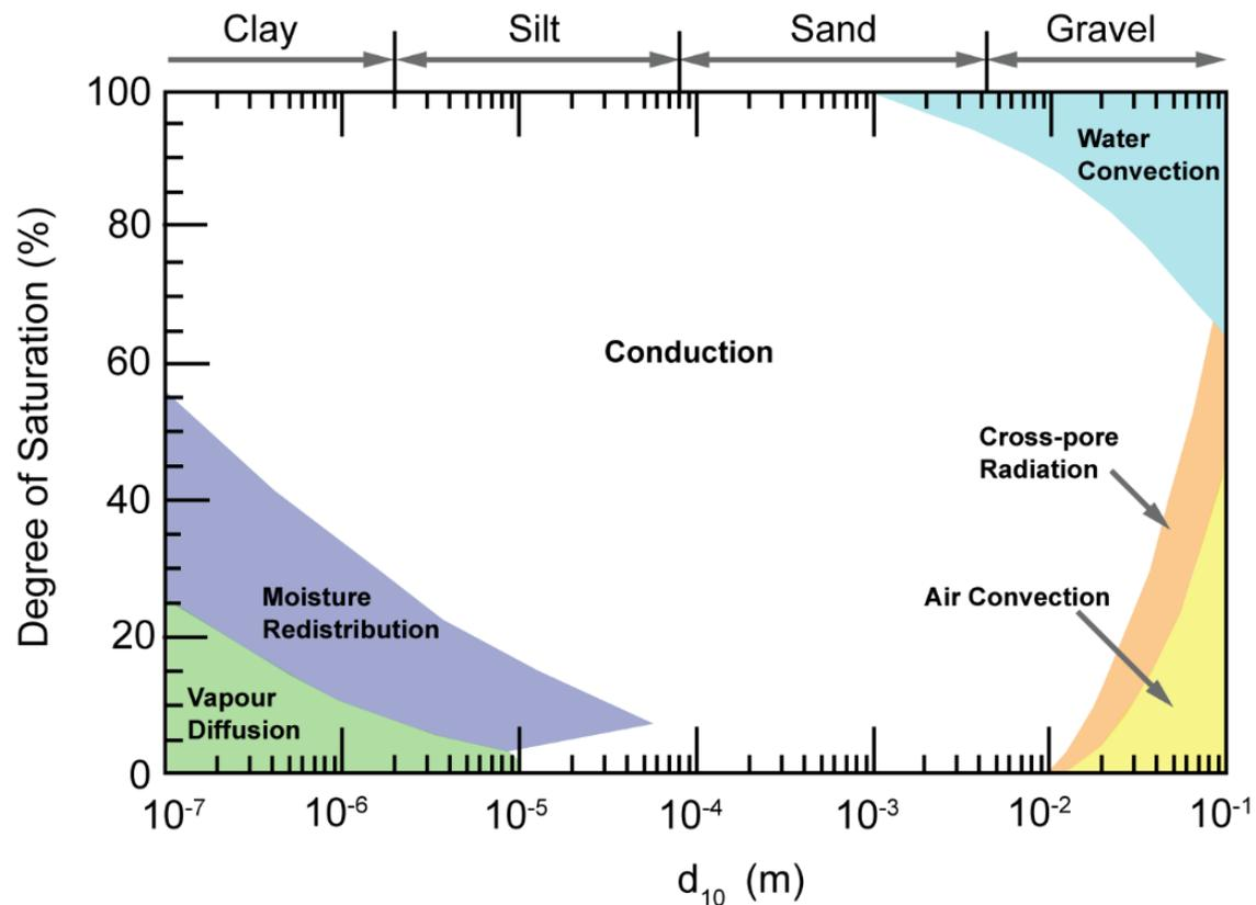
Figure 2. Heat transfer mechanisms for soils based on  $d_{10}$  particle size and degree of saturation (modified from Johansen 1975).
