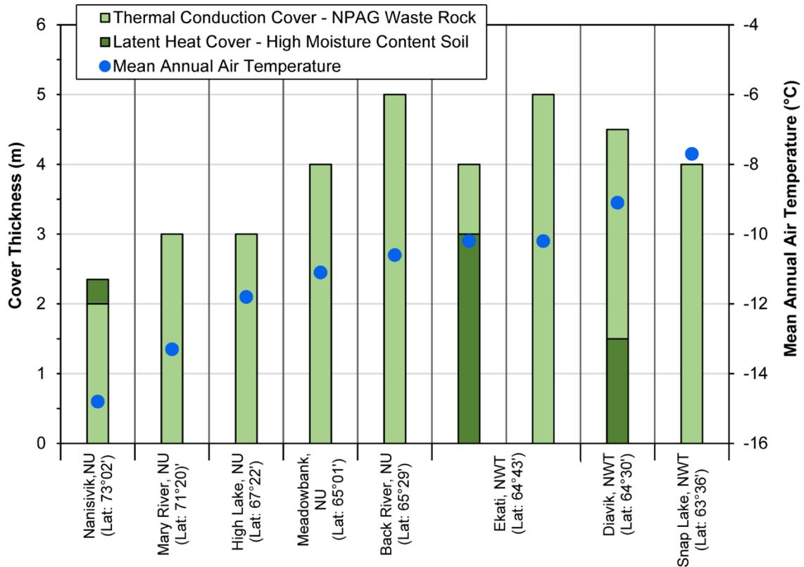
Figure 5. Summary of thermal conduction covers and latent heat covers for waste rock facilities in Canada.
