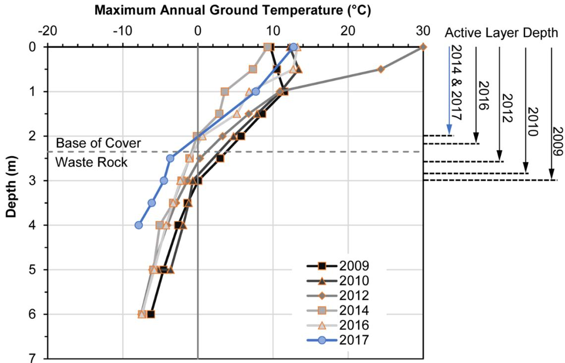
Figure 6. Measured ground temperature from mid-August and estimated active layer depth for the Nanisivik West Open Pit Waste Rock Thermal Cover. Ground temperature data reproduced from BGC (2018).
