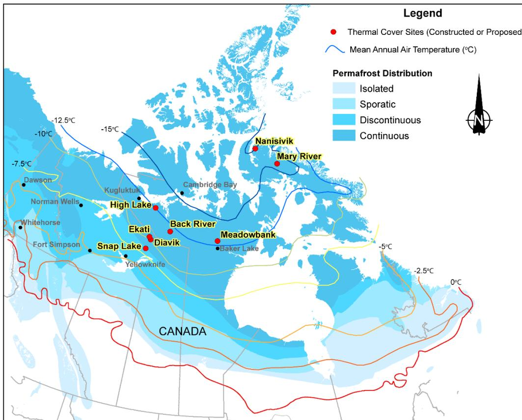
Figure 4. Thermal covers constructed or proposed for closure of waste rock facilities in Canada.
