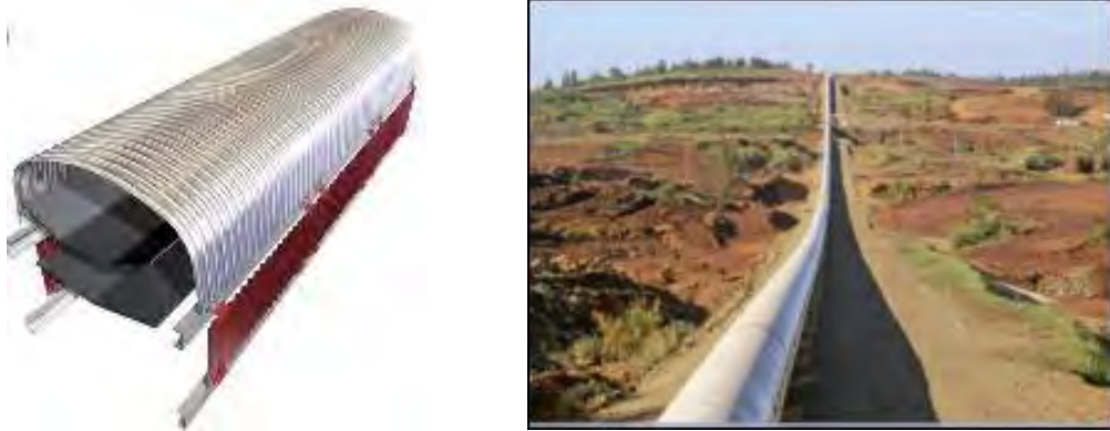
Figure 5.5.5: Images illustrating the enclosure of a conveyor (source www.capotex.com ).
