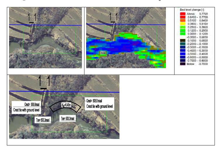
**Zone 1\_2** This area is within the servitude and has unstable banks. Due to the bedrock at the location, the banks do not need protection and the servitude seems incorrect.
