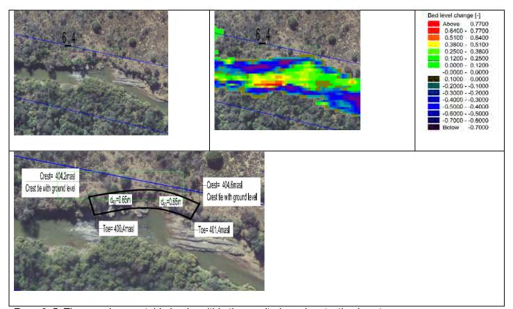
**Zone 6\_5** The zone has unstable banks within the servitude and protection is not necessary.
