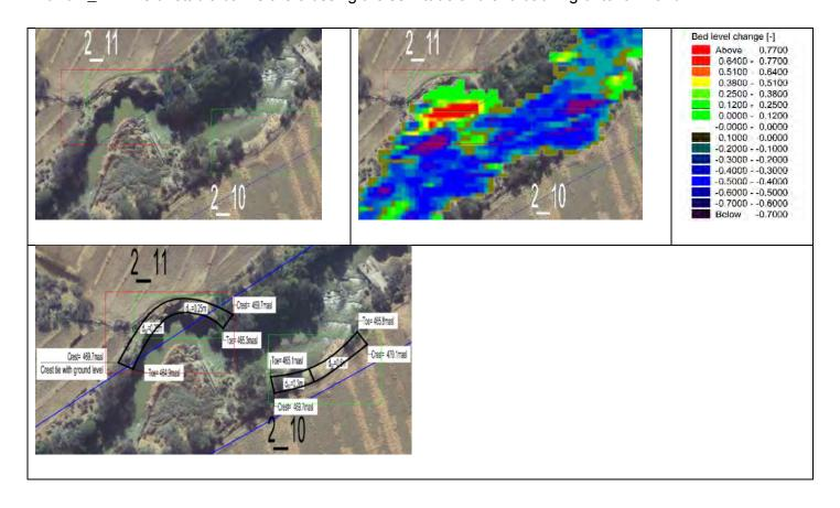
**Zone 2\_12 and 2\_14** This area is within the servitude but encroaches farmland. An old weir diverts water inducing erosion. Protection does not seem necessary.
