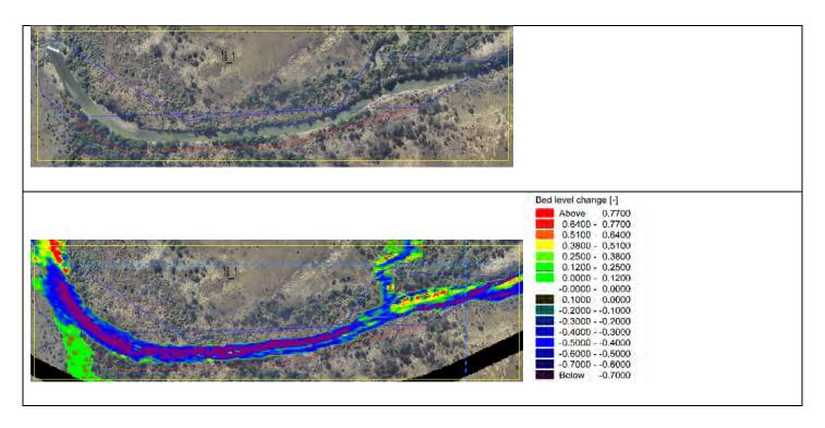
**Zone 10\_2** The zone has unstable banks within the servitude. Protection in this area is not necessary.
