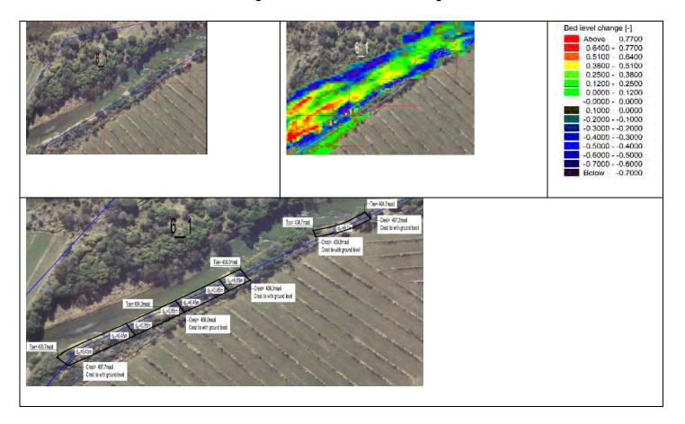
**Zone 6\_2** The zone has banks within the servitude. Upstream tributary flow induces the erosion and protection will constrict the flow thus not necessary.
