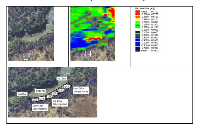
**Zone 4\_5 and 4\_6** Flow in this area is on a wide floodplain and erosion induced by a tributary thus protection is deemed not necessary.
