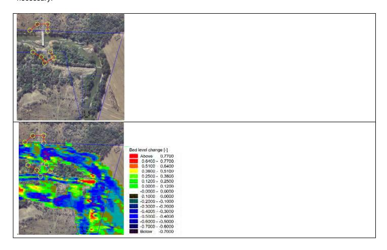
**Zone 5\_6** The zone has banks within the servitude. Flows are wide on the floodplain and protection not necessary.
