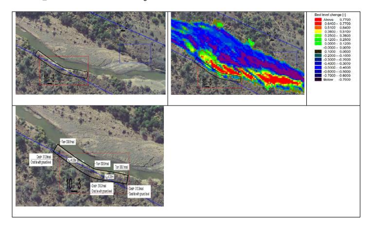
**Zone 10\_4** The zone has banks within the servitude. Upstream tributary flow induces the erosion and protection will constrict the flow thus not necessary.
