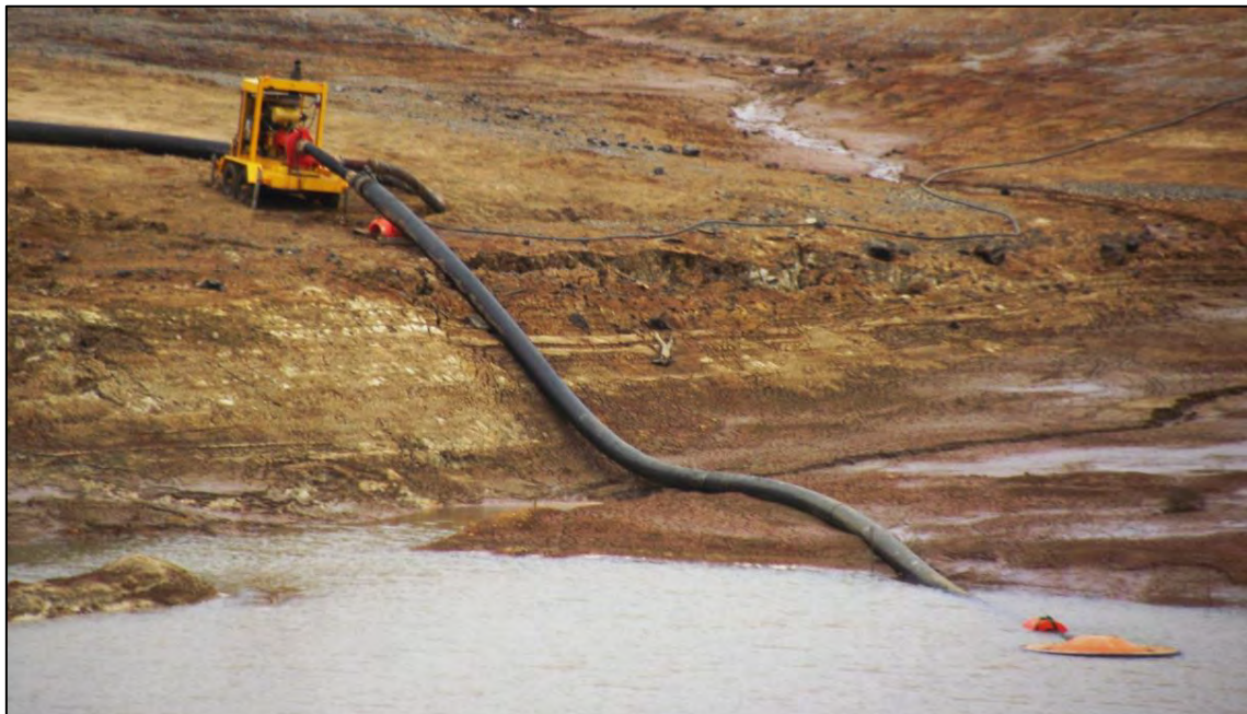
FIGURE 14-4: TURRET SYSTEM POSITIONED IN THE SUPERNATANT WATER CONNECTED TO AN EXTERNAL PUMP
