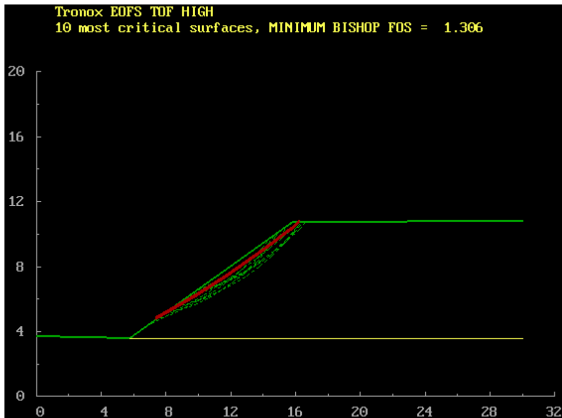
Figure 2-2: Stability Run Depicting Higher Range \phi (42°)
