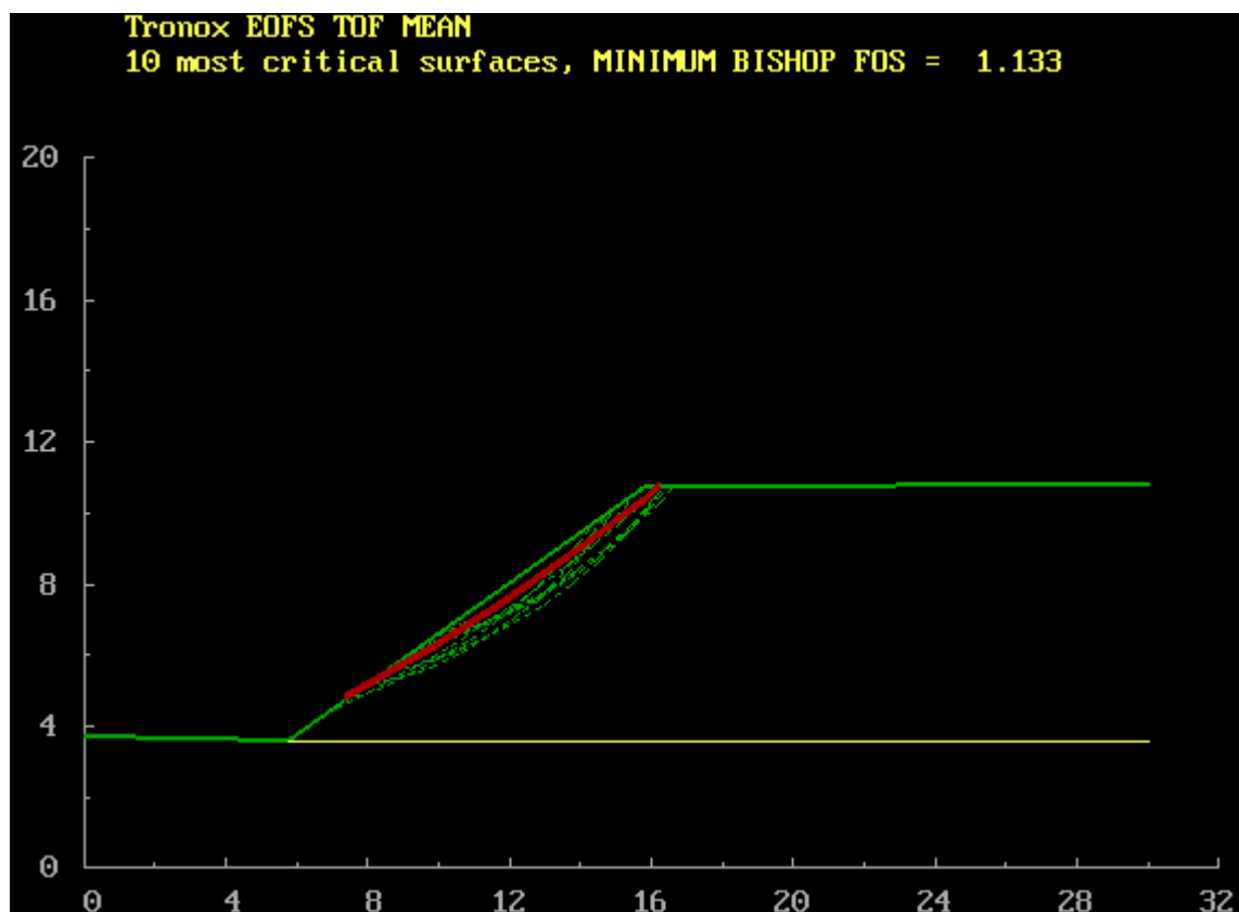
Figure 2-3: Stability Run Depicting Mean Range \phi (38°)
